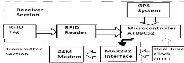
Figure- 6. Typical RFID rail tracking system a) RFID and GPS based receiver section b) GSM based Transmitter Section
