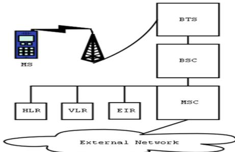
Figure-3. GSM Architecture and Working of GSM Networks
