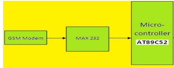
Figure-5. Interfacing of GSM with AT 89c52 through Max232
