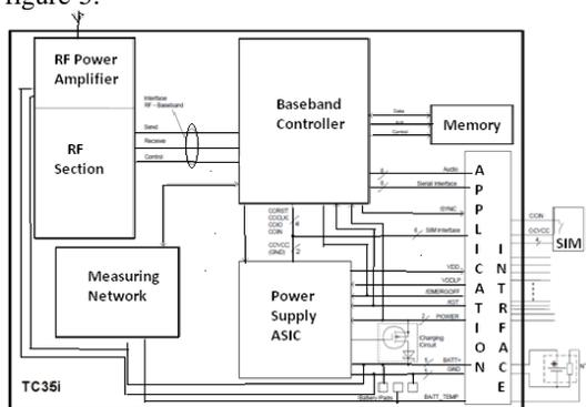
Figure-5. Block diagram of GSM TC35i
