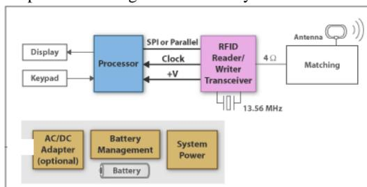
Figure-1. Block diagram of RFID system.
