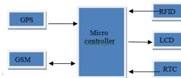
Figure-4. Interfacing of Peripherals with Microcontroller
