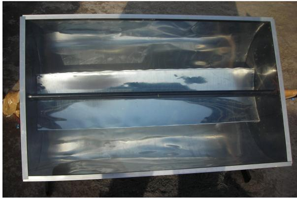
**Picture 1.** Photographs of multifocus glass covered paraboloidal solar air collector.
