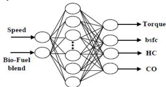
Figure 6. Configuration of Multilayer Neural Network for predicting engine parameters
