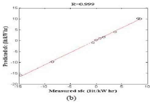
Figure 8. The predicted output vs. the measured values, (a) engine torque (b) SFC
