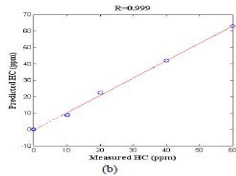
Figure 9. The predicted output vs. the measured values, (a) CO (b) HC
