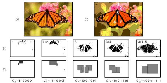
FIGURE 2. (a) Butterfly color image, (b) processed color image with 30 colors, (c) pixels from image (b) belonging to color set  $C_i$ , (d) minimum bounding rectangles (MBRs) for extracted regions used to index the image collection.
