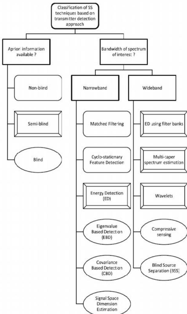
Fig.1 Spectrum Sensing Techniques based on Primary transmission detection [10]
