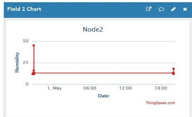
**Figure 10: Humidity at node 2 when there is no leakage**
