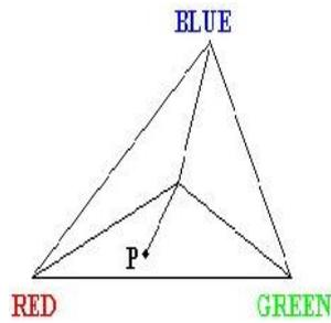
In Figure 2.2 (i) the obtainable HSV colors lie within a triangle whose vertices are defined by the three primary colors in RGB space. The hue of the point **P** is the measured angle between the line connecting **P** to the triangle center and line connecting RED point to the triangle center.
