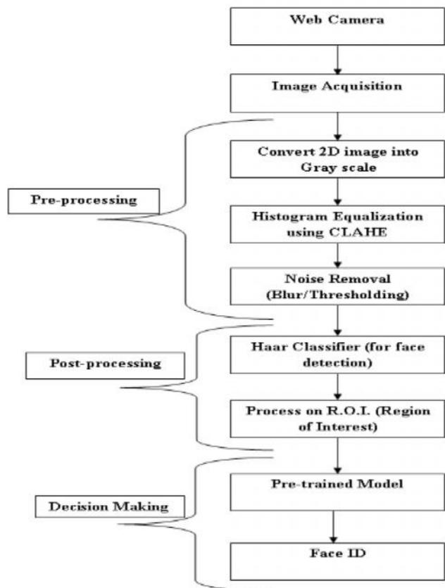
Fig.3. Working Flowchart of System
