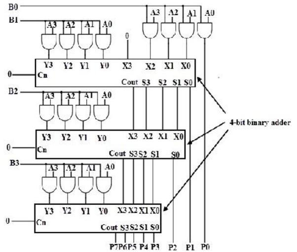
c) Generalized CMOS design for 4-bit multiplier
