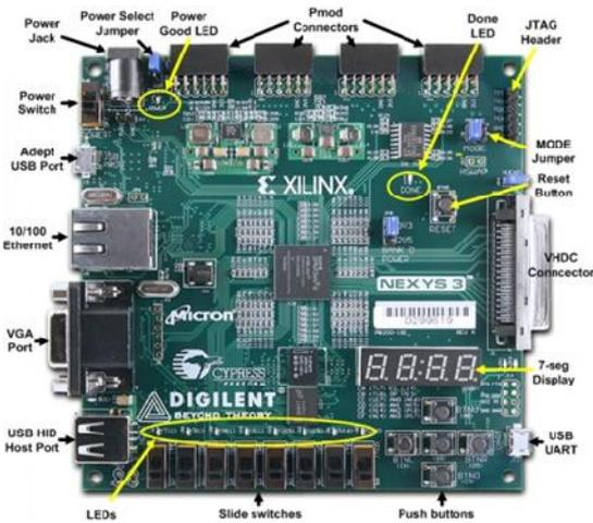
Fig. 2. Xilinx Nexys 3 FPGA board
