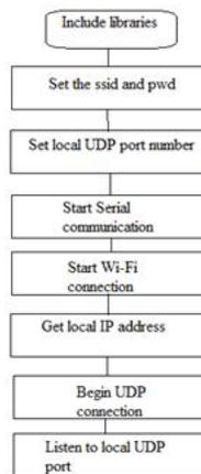
Fig. 5. Receiver NodeMCU flowchart
