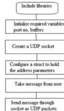
Fig. 7. Flowchart for socket programming (Linux)
