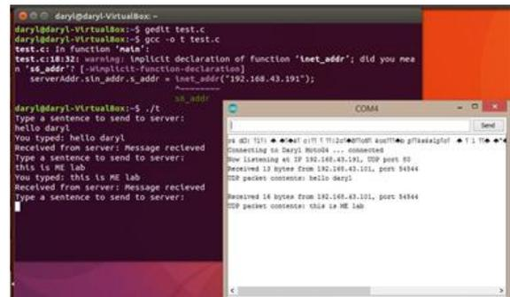
Fig. 8. UDP packet from PC to NodeMCU
