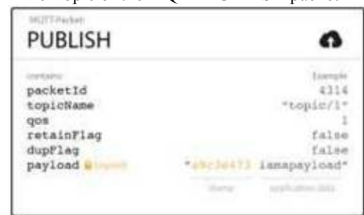
Fig: 6.1 MQTT publish packet
