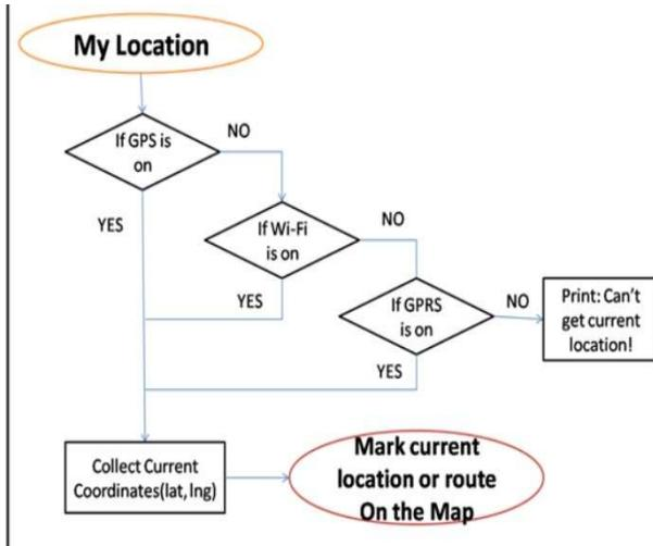
**Figure.(01)** showing the working of GPS
