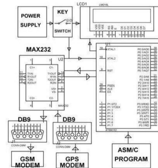
**Figure.(04)** Shows the block diagram of vehicle tracking and locking system based on GSM and GPS technology.
