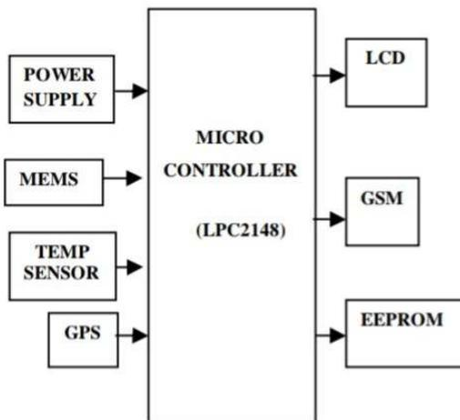
**Figure.(03)** Showing the intelligent vehicle control and monitoring using GSM and GPS.
