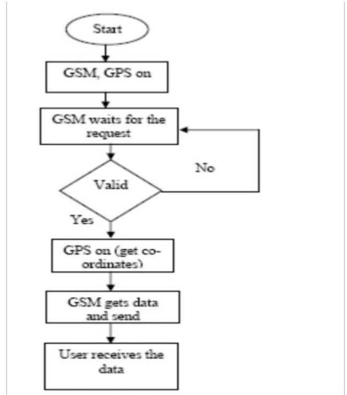
**Figure.(06)**shows the flowchart of vehicle tracking system.
