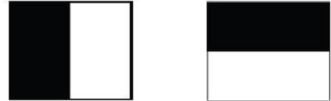
Fig. 2. The Haar wavelet filters used to describe the interest points.
