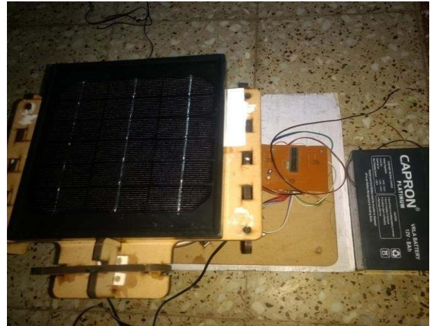
Fig. 5 Experimental setup of Dual Axis Solar Tracking System
