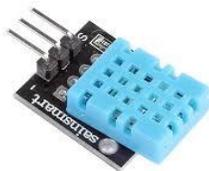
The DHT11 is a basic, low-cost digital temperature and humidity sensor. It gives out digital value and hence there is no need to use conversion algorithm at ADC of the microcontroller and hence we can give its output directly to data pin instead of ADC. It has a capacitive sensor for measuring humidity. The only real shortcoming of this sensor is that one can only get new data from it only after every 2 seconds. [4]
