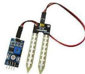
Soil moisture sensor is a sensor which senses the moisture content of the soil. The sensor has both the analog and the digital output. The digital output is fixed and the analog output threshold can be varied. It works on the principle of open and short circuit. The output is high or low indicated by the LED. The sensor is platinum coated to make the efficiency high. The range of sensing is also high. [1]
