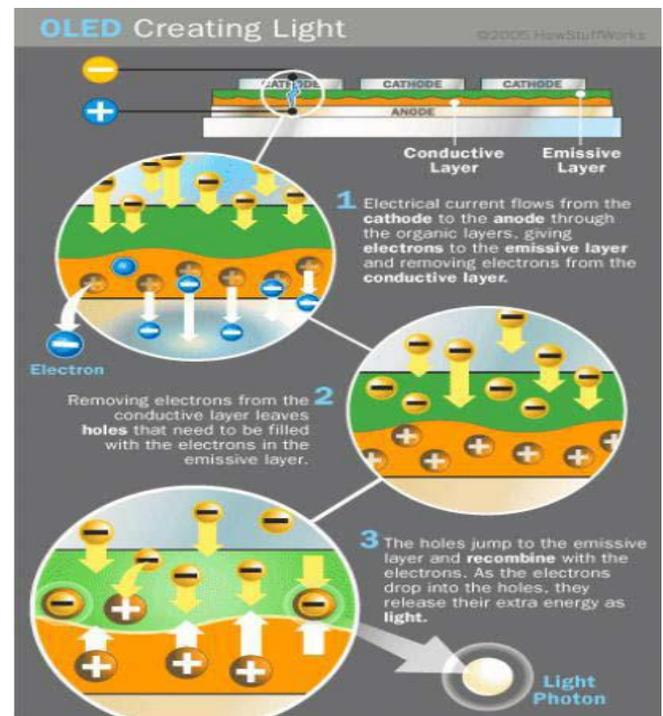
Fig. 4. Working principle of OLED
