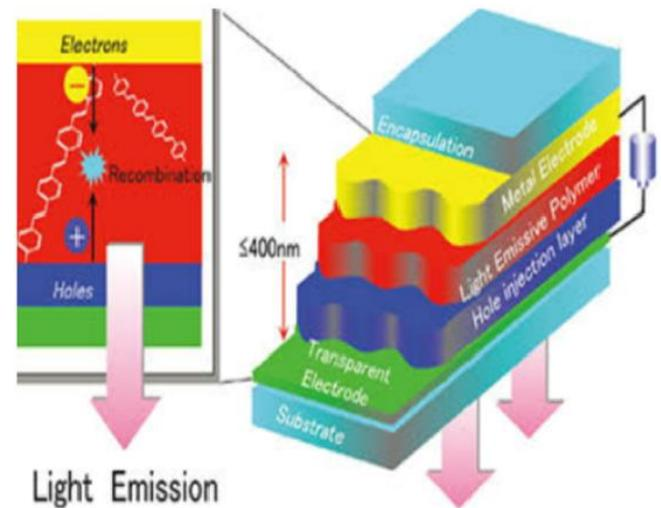
Fig. 7. Polymer material OLED
