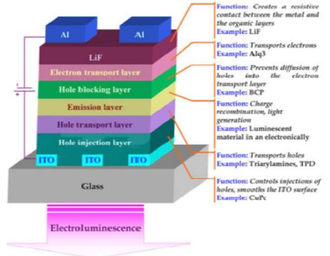
Fig. 6. Small molecule material OLED
