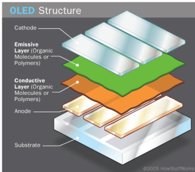
Fig. 3. Structure of OLED
