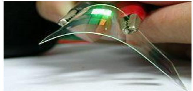
Fig. 2. Demonstration of a flexible OLED device
