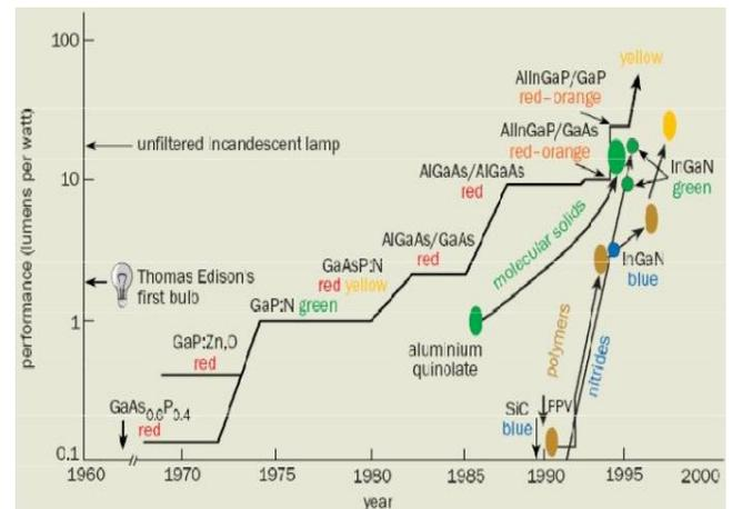
Fig. 1. OLED progress (Originally from Sheats et al. Science 273, 884, 1996)
