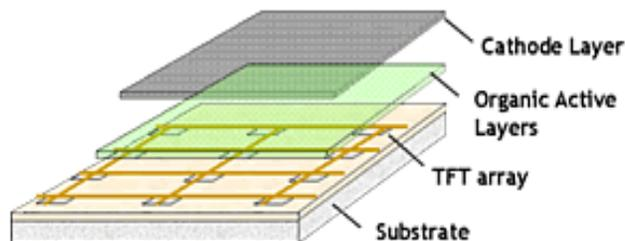
Fig. 9. Active Matrix OLED (AMOLED)
