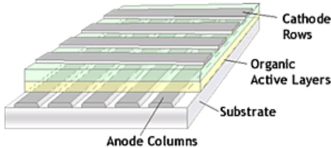
Fig. 8. Passive Matrix OLED (PMOLED)
