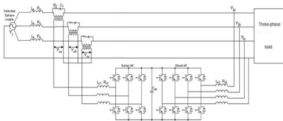
**Figure 4. Detailed configuration of UPQC**
