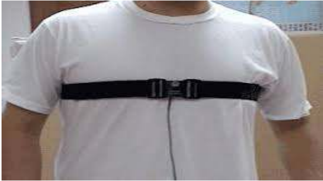
Figure 3: Respiratory belt for breath analysis
