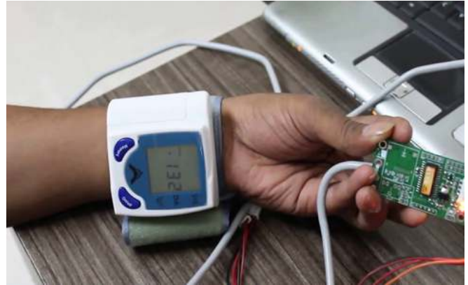
Figure 4: Blood pressure sensor unit to wrist for measuring systolic and diastolic
