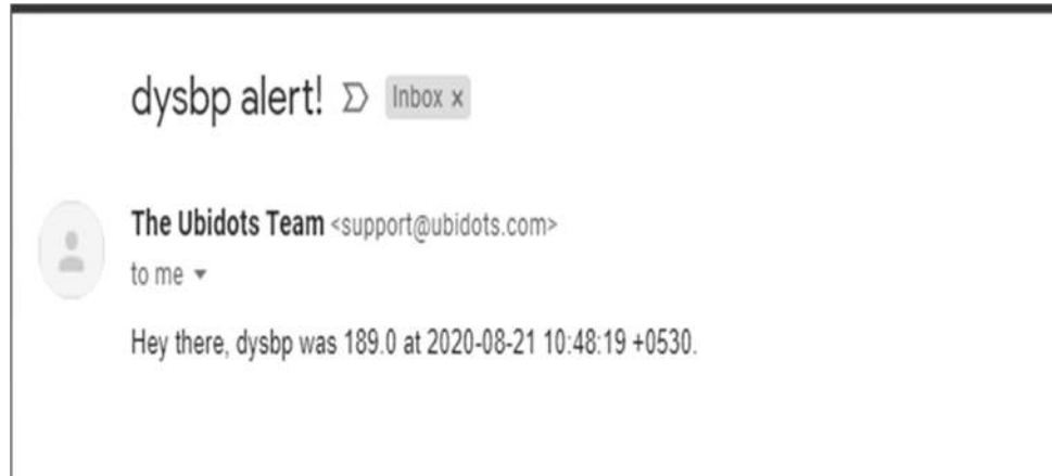
Figure 8: Alert On email after value exceed some threshold value set in event generation
