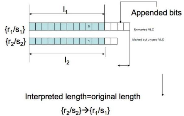
Fig. 3. Mapped VLC appears as another VLC of the same length. The new size S<sub>2</sub> must be remapped to S<sub>1</sub> to maintain synchronization. Also r<sub>2</sub> = r<sub>1</sub>.
