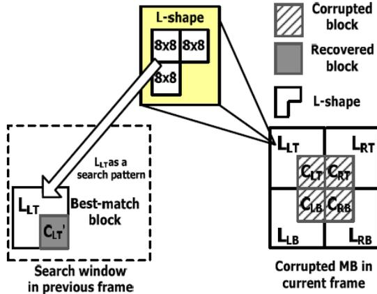
Fig 6. The illustration of corrupted MB in the block matching principle with the L-shape as a search pattern.
