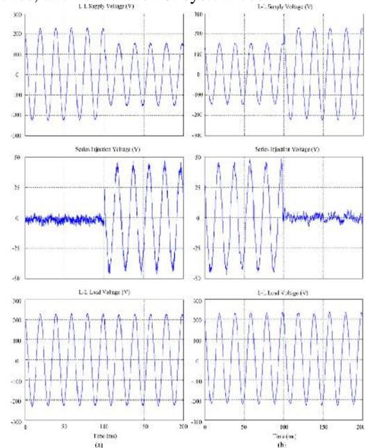
**Fig. 4.4** Experimental supply, series injection, and load voltages during (a) normal-to-sag and (b) sag-to-normal transitions
