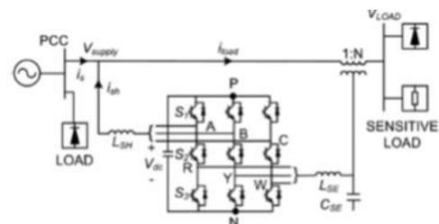
**Fig. 1.2 Representation of Integrated Nine Switch Power Conditioners**
