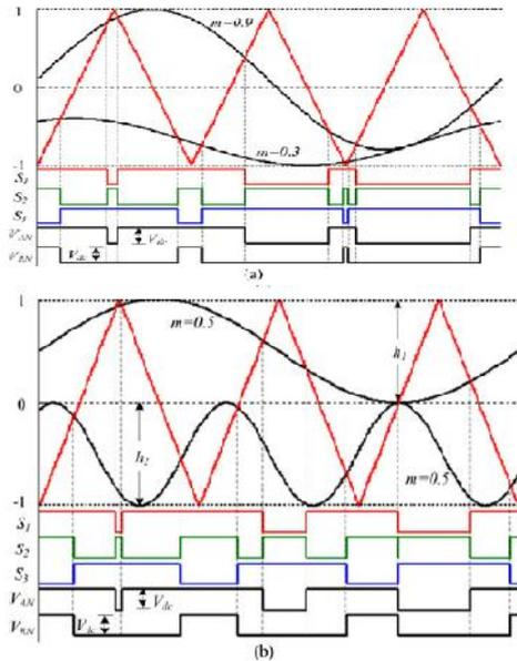
**Fig. 2.2.1** Arrangements of references having (a) the same frequency but different amplitudes, and (b) different frequencies but the same amplitude.
