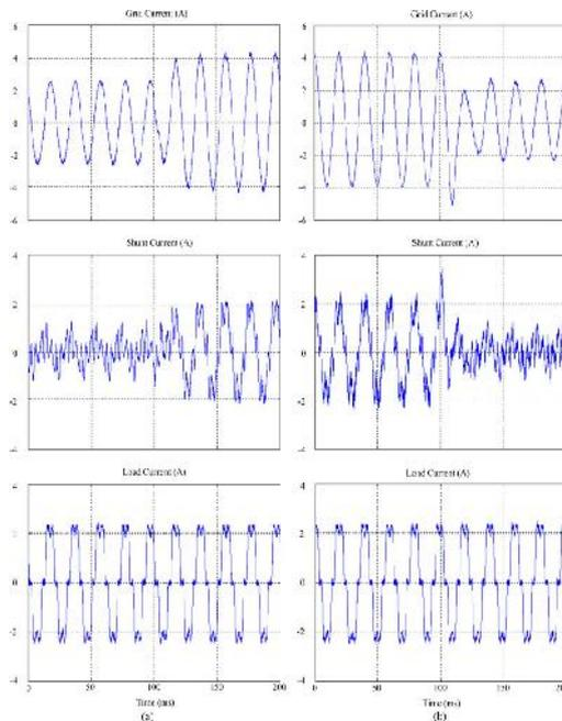
**Fig. 4.5** Experimental grid, shunt injection, and load currents during (a) normal-to-sag and (b) sag-to-normal transitions
