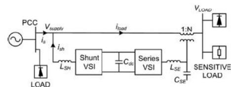
**Fig. 1.1 Representation of Back to Back Converter**
