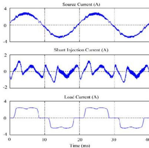
**Fig. 4.3** Experimental source, shunt injection, and load currents captured during normal power conditioning mode
