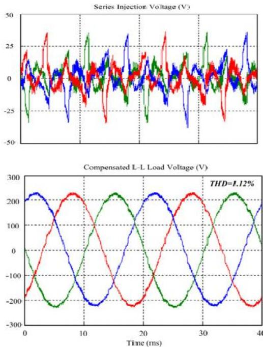
**Fig. 4.2** Experimental supply, series injection, and load voltages captured during normal power conditioning mode
