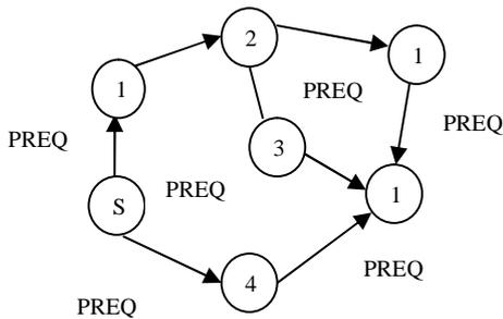
Fig1: Discovery phase 1: the path requesting phase(S-sender, R-Receiver)
