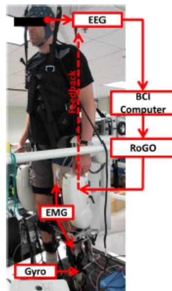
Fig.1. The experimental setup showing a subject suspended in the RoGO, while surface EMG electrodes, a gyroscope and donning an EEG cap on the left leg. A monitor, placed in front of the subject at eye-level, presented instructional cues.
