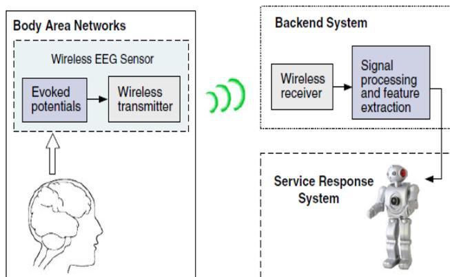
Fig.2. Architecture of a BAN based wireless BCI system
