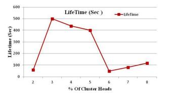
Figure 4: Analysis of lifetime by varying no. of cluster heads
